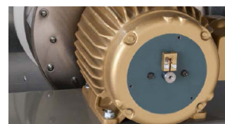
Bottom photo shows Baldor shaft grounding brush without the protective cover.
