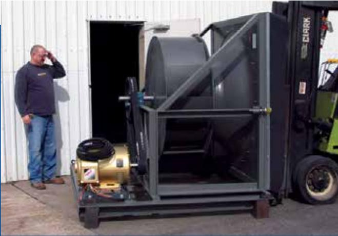
Don't let replacement fan size prevent you from upgrading your air system. FANWALL cells fit through standard width doors and can be stacked in any configuration to fill the air tunnel. At the right is a timeline from an actual retrofit job which converted a single fan to a four-cube FANWALL array. The time shown not only includes the fan retrofit work, but also changing the unit from a blow-thru to a draw-thru arrangement.
